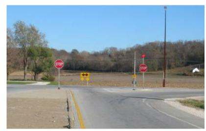
Photo 3 - Example of a supplemental STOP sign mounted on left in a splitter island.
