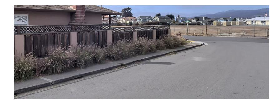
10.Curb ramps on 3rd and Central encourage diagonal crossing, need a safer way to cross
