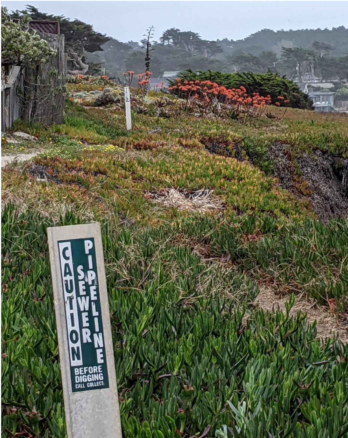
Picture 11: Slip on active scarp visible as cut in edge of cliff. Notice the sewer Caution markers. This sewer was re-aligned about 10 feet inland after this slip several years ago which caused a pipe failure.
