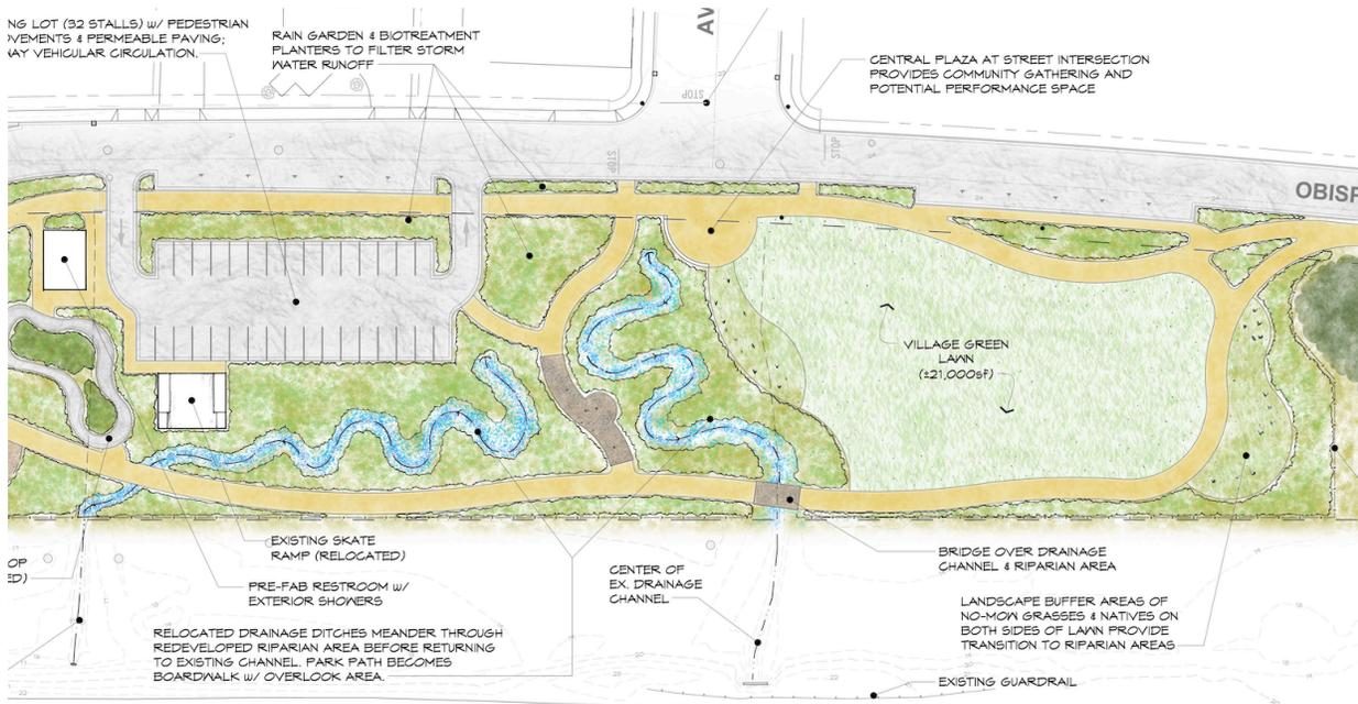
The existing, deeply-incised central drainage channel that extends from Avenue Portola is relocated from its current location slightly to the north, its channel both widened and realigned to increase sinuosity, allowing for more stormwater percolation and filtration. The area surrounding this meandering drainage will be a much more robust and dynamic riparian zone, with opportunities for educational signage and viewing/seating areas.
