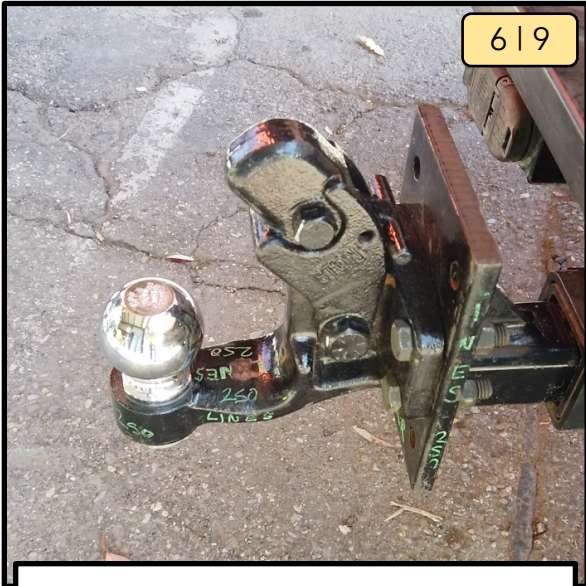
Inspect the hitch/pintle/ball to ensure they are the correct fit and are undamaged.
