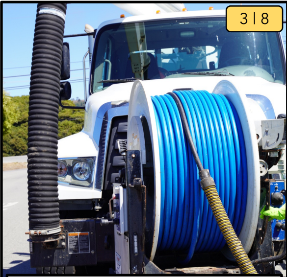
Purge all excess water from the hose to reduce its weight when carrying it to the manhole.
