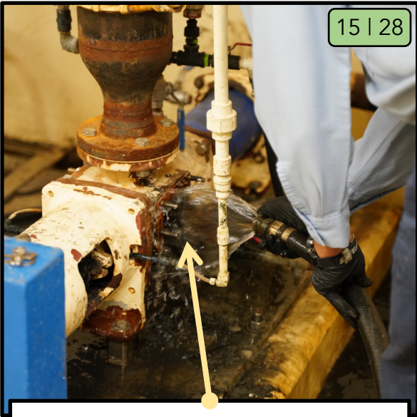
Spray inside the compartment to clean out any excess discharge.
