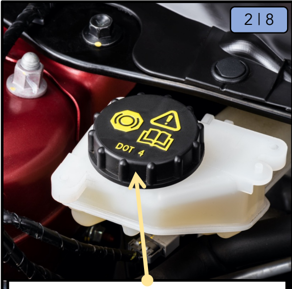
Check if the brake fluid is at an appropriate level. (Not applicable to vehicles with air brakes.)
