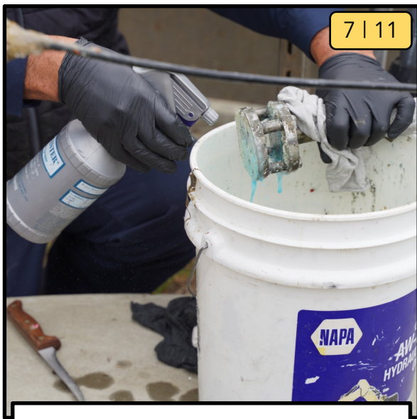
Continue spraying with the degreaser until the transducer is clean.
