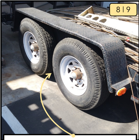
Inspect the Springs / Axle for damage.
