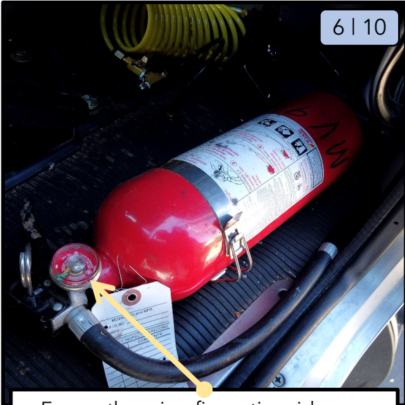
Ensure there is a fire extinguisher on board and that its pressure gauge is in the "green". Check to make sure it is up to date on its monthly inspections.
