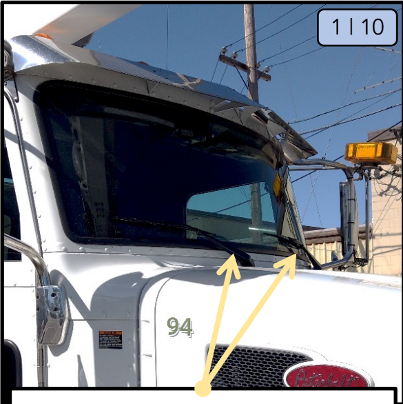
Inspect the windshield wipers, ensure they are functioning and undamaged.
