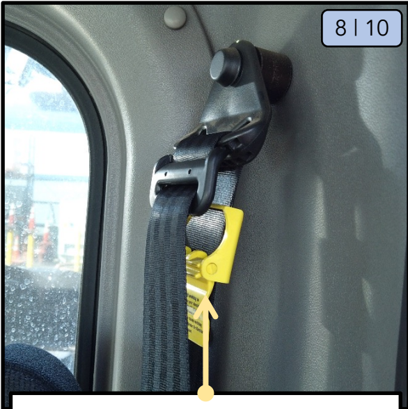
Inspect the seatbelts for damage and make sure their emergency locking mechanism is functioning.
