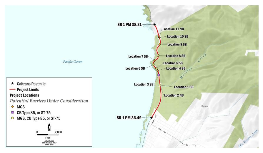
Figure 1-4 Barrier Types Under Consideration by Location
