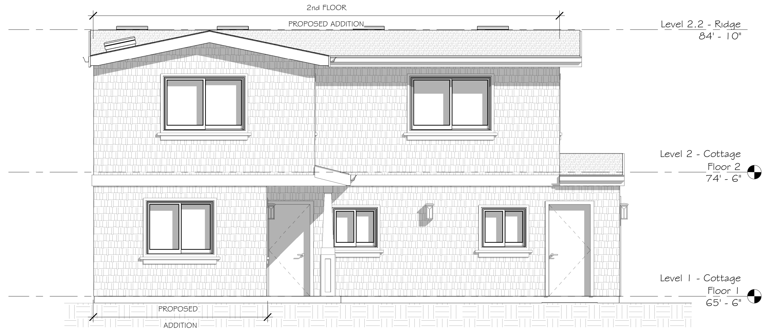
④ Elevation - South (Left) Proposed 1/4" = 1'-0"
